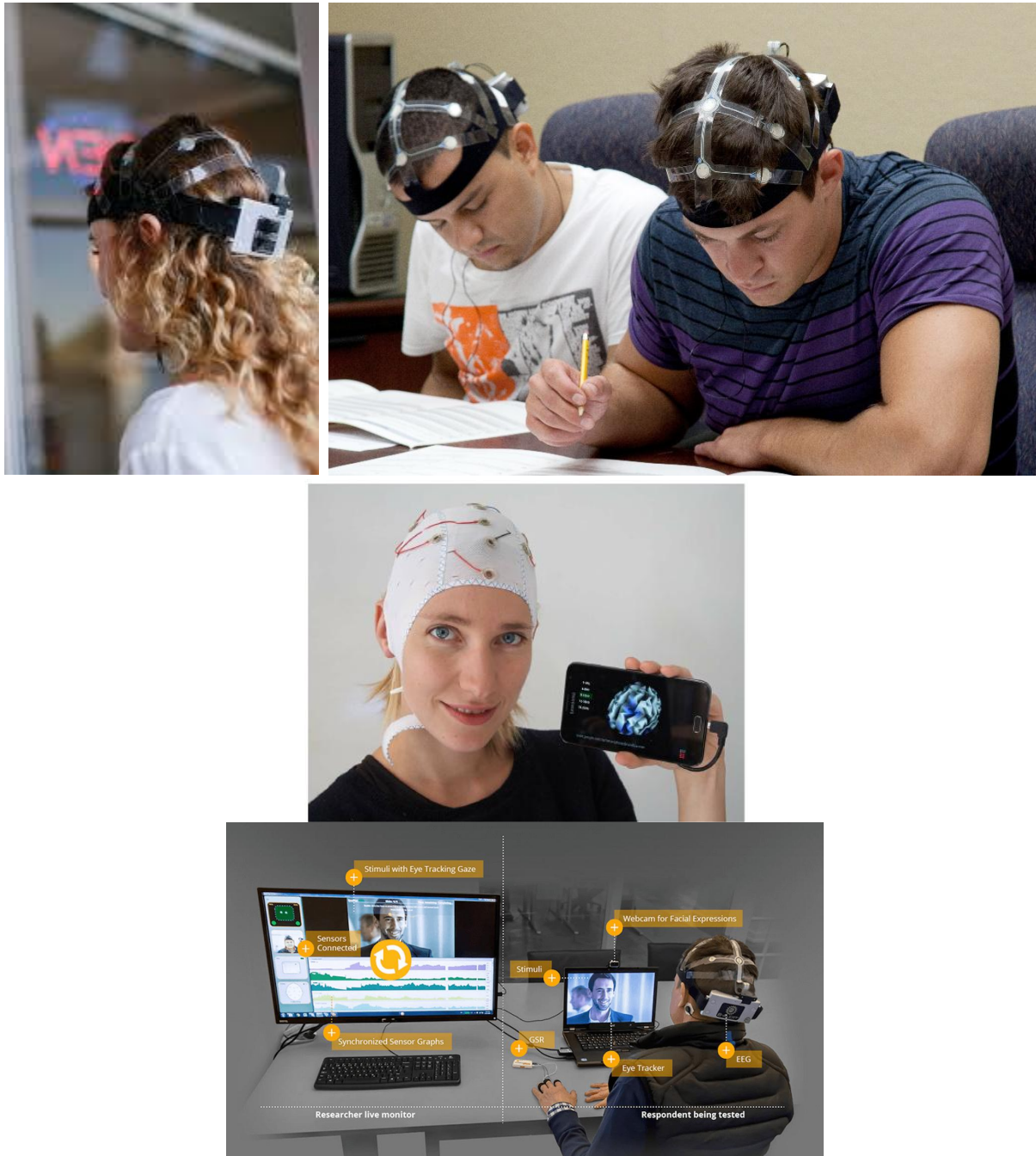
Figure 1. Mobile and portable EEG equipment
